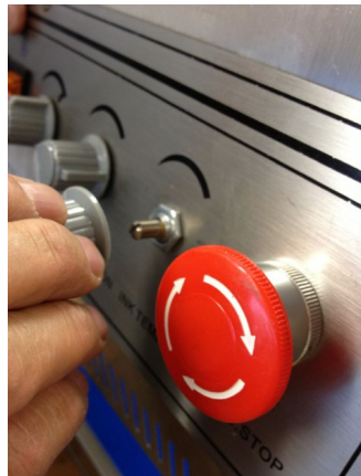
Figure 31. Remove Ink Temperature Knob
