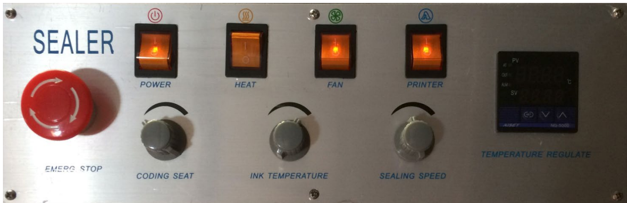
Figure 7. Control Panel of FRM-1010
