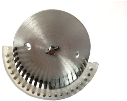
Figure 16. Ensure two holes and pins line up with the base
